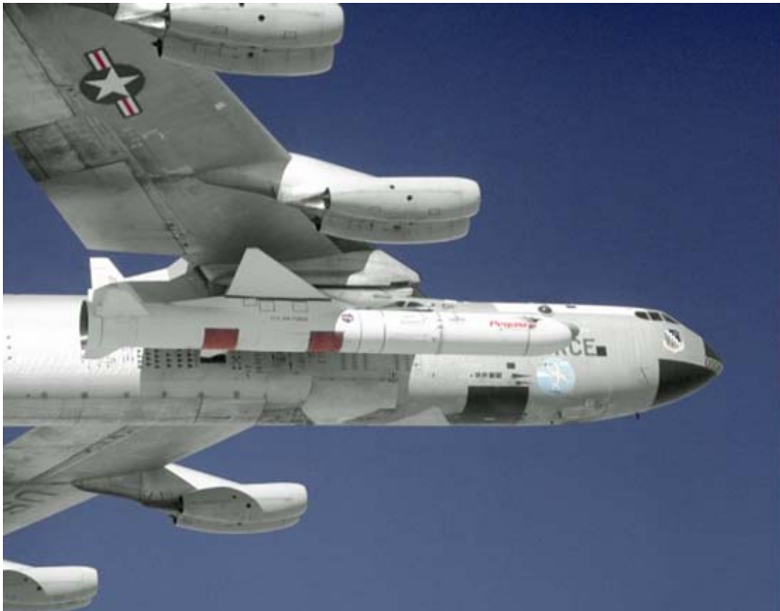
Figure 3 - The American rocket Pegasus under a B-52. Pegasus is here used to place a satellite into orbit from an airplane (Photo by NASA)
